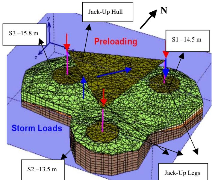
Figure 6, 3D FE structure-foundation model, final gravel banks
