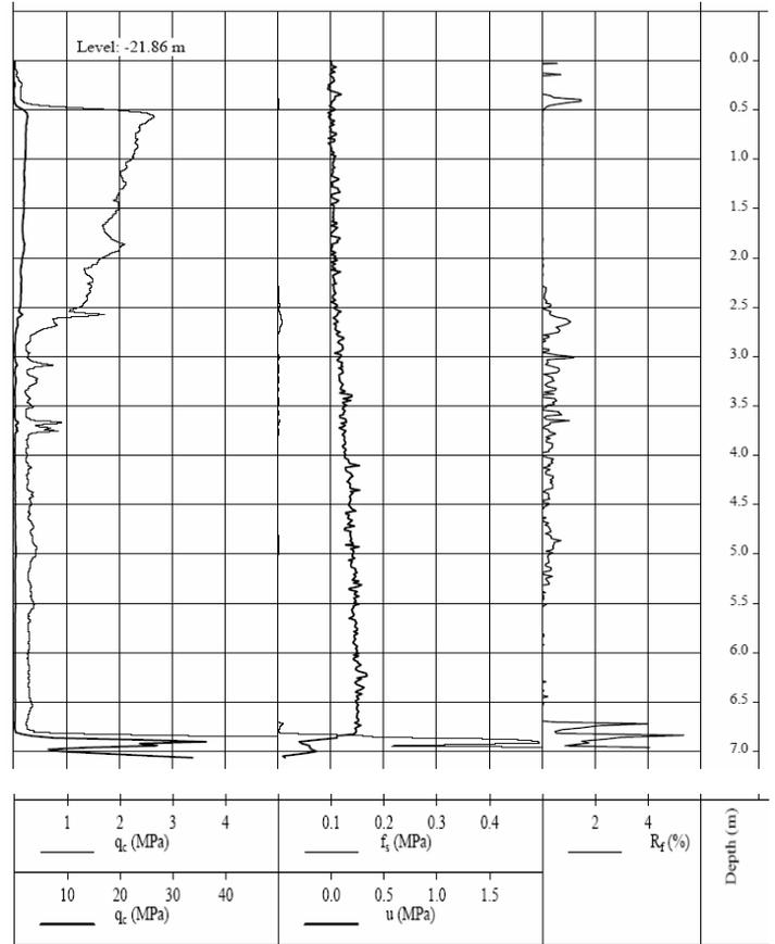
Figure 3, PCPT profile at S1 location
