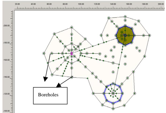
Figure 5, 3D FE structure-foundation model, 2D build-up, horizontal plane at S1 level,  $-14.5 \text{ m}$
