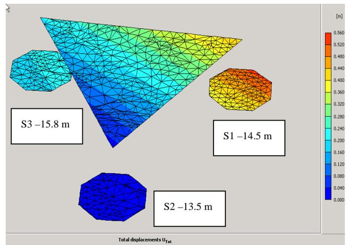
Figure 11, Preloading phase, structure total displacements (only plate elements shown)
