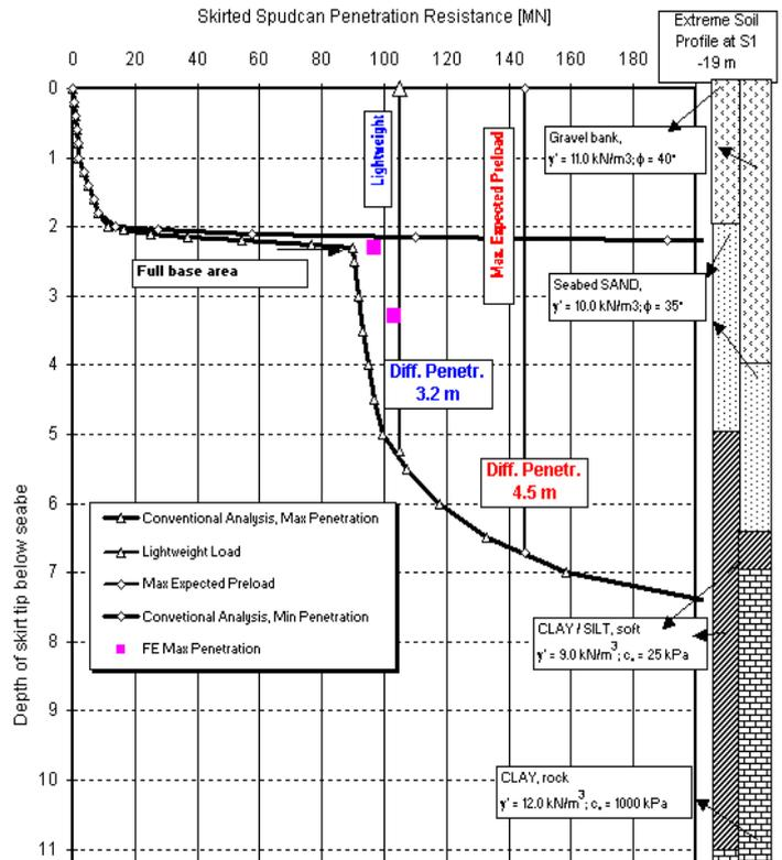
Figure 4, Conventional skirted spudcan differential penetration analysis, S1 extreme soil conditions, and gravel bank at  $-19$  m
