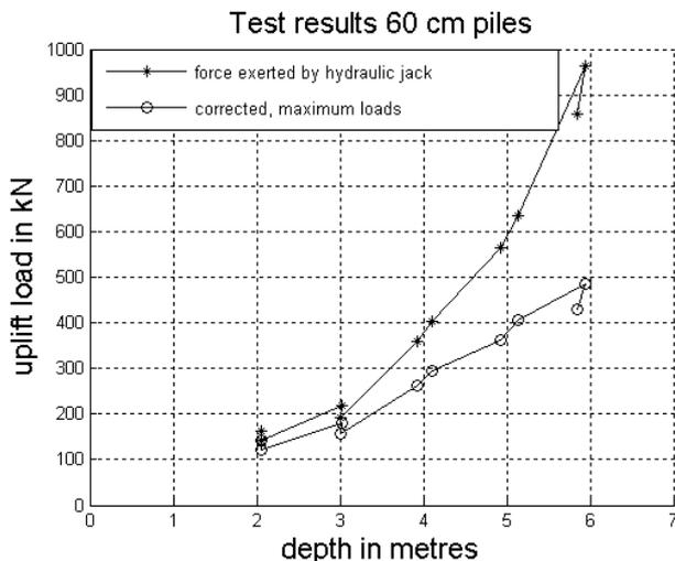
Figure 4. Test results of 60 cm piles
