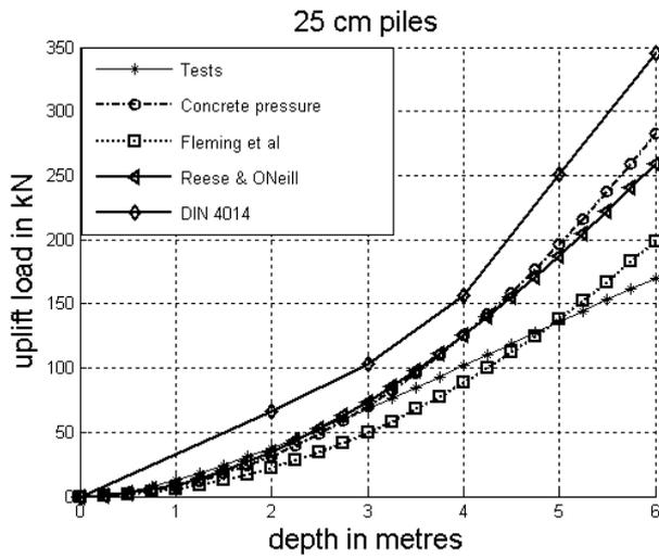
Figure 7. 25 cm piles in dense sand.
