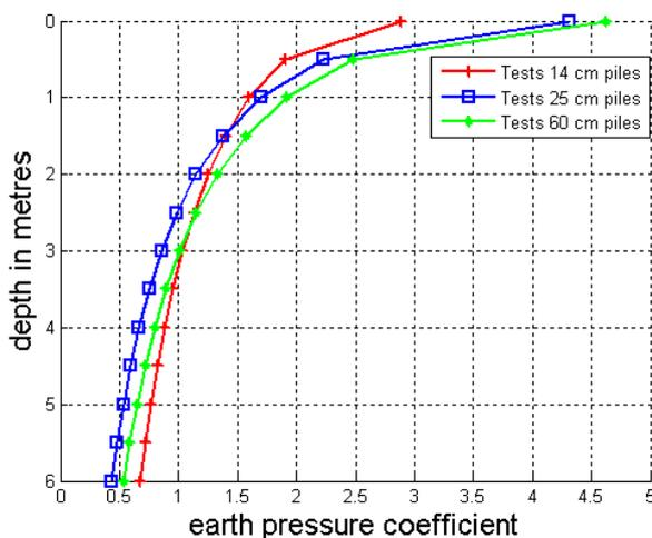
Figure 5. Variation of earth pressure coefficient  $K$ .
