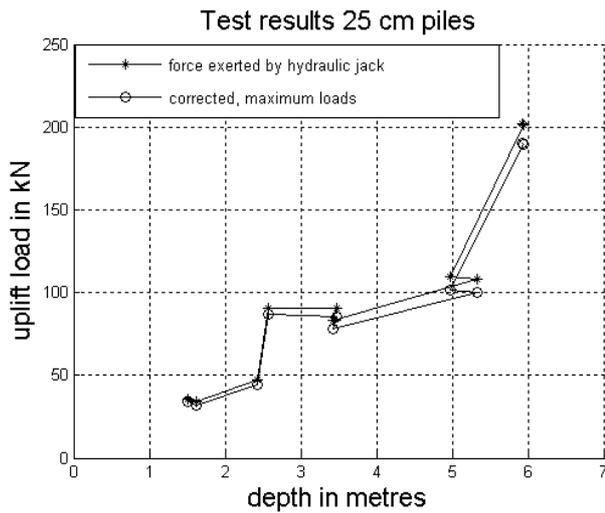
Figure 3. Test results of 25 cm piles
