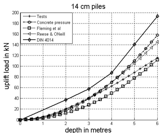
Figure 6. 14 cm piles in dense sand.
