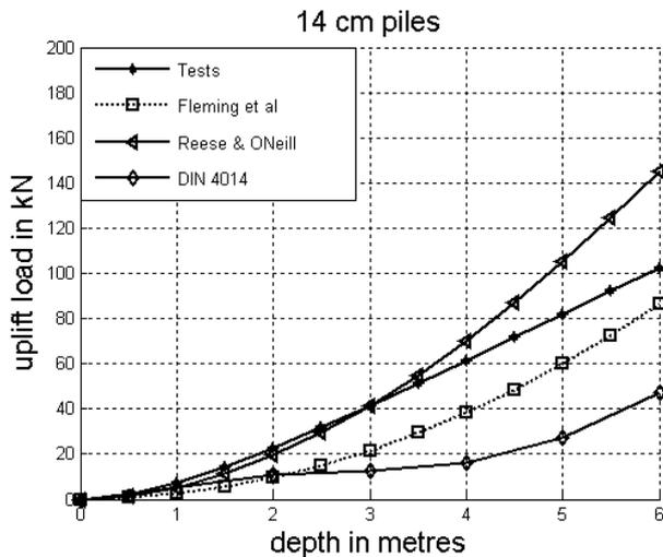
Figure 9. 14 cm piles in loose sand.
