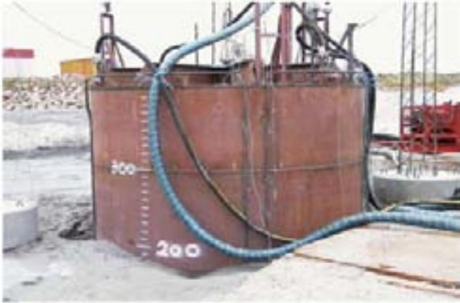
Figure 11. The critical suction has been achieved and soil failure by piping has occurred.
