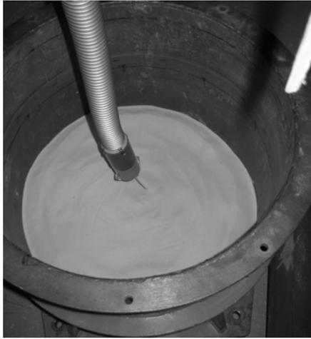
Figure 5 Spot pouring hopper for preparation of sand samples.
