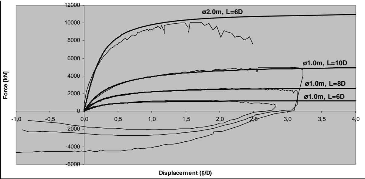
Figure 10 Load-displacement curves for pile tests.
