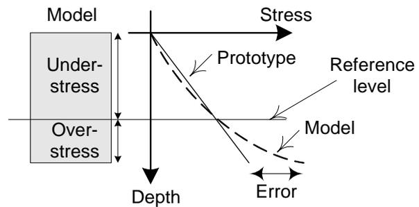
Figure 2 Comparison of vertical stress variation in centrifuge model and corresponding prototype.
