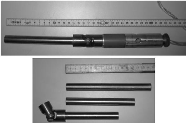
Figure 9 Bending beam load cell and pile(s).
