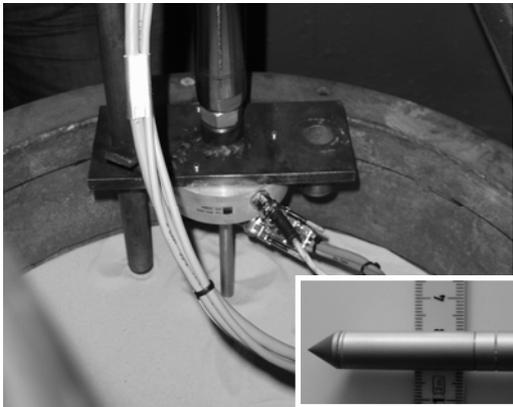
Figure 6 Mini cone penetrometer
