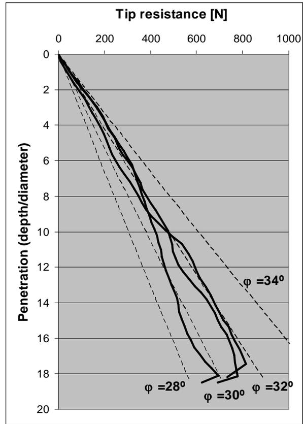
Figure 7 Results from cone penetration test in medium dense sand ( $I_d = 0.55$ ). Test is at 61g and the results are not scaled.
