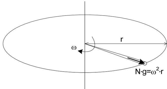
Figure 1 Acceleration by rotation
