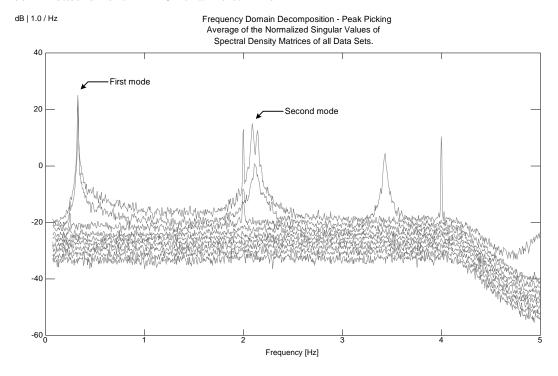
Figure 20 Frequency plot for measurement "21mar05" (without wings).
