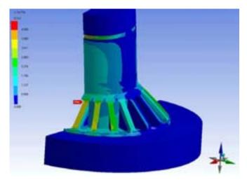
Figure 10. Finite Element model for detail design.
