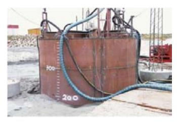
Figure 11. The critical suction has been achieved and soil failure by piping has occurred.
