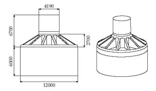
Figure 3. Dimensions of the prototype. Dimensions in mm.
