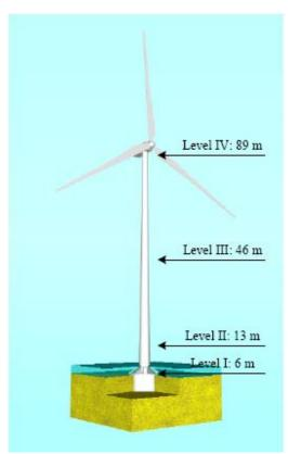
Figure 16. Sensor positions in tower and foundation.
