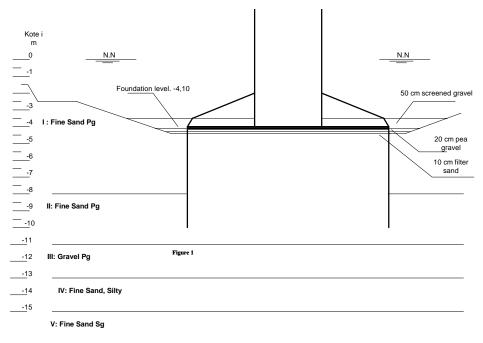
Figure 5. Sketch of the installed bucket foundation.
