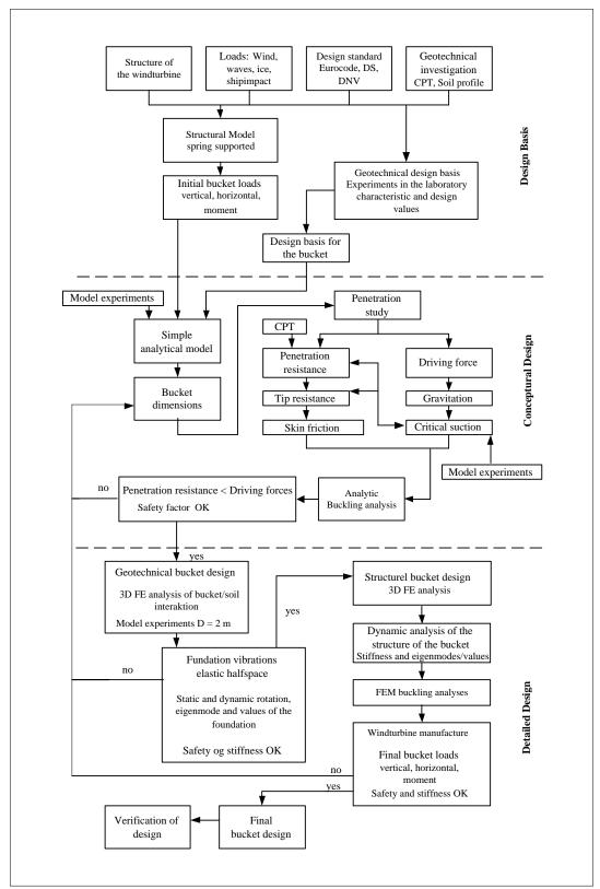
Figure 9. Design Chart for bucket foundations.
