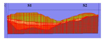
Figure 7, Cross section profile North – South at S1 across the 3D FE model (not to scale)
