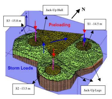
Figure 6, 3D FE structure-foundation model, final gravel banks
